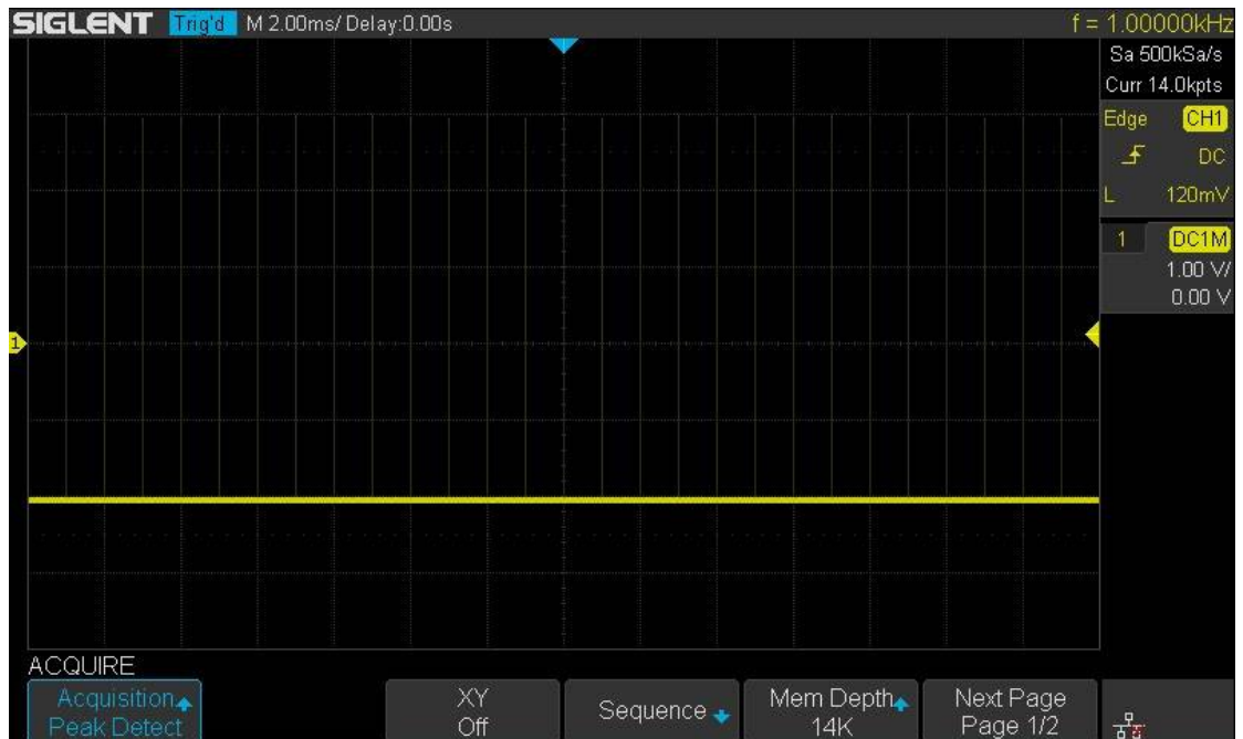
Figure 24 Pulse With 0.1% Duty, Peak Detect Mode
